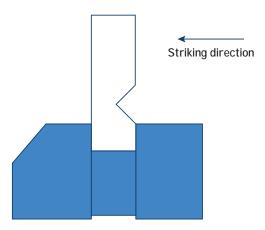
Charpy impact testing also utilizes a pendulum to impact the piece. Yet, the orientation of the piece is horizontal and the impact is opposite the notch side. This test simulates a high speed flexural test (three point bend) of the material. Charpy impact is particularly valuable in measuring the effect of micro cracking, flow and weld lines on the parts toughness.
