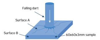
There are part attributes that influence impact strength of the tested part. A molded part with stress concentrations, such as voids or sharp corners, may reduce impact strength. Thin walls have less volume to absorb and dissipate energy, thus are more brittle than heavy cross sections. Part exposure to environmental stress, temperature, UV and chemical exposure can weaken impact resistance.
